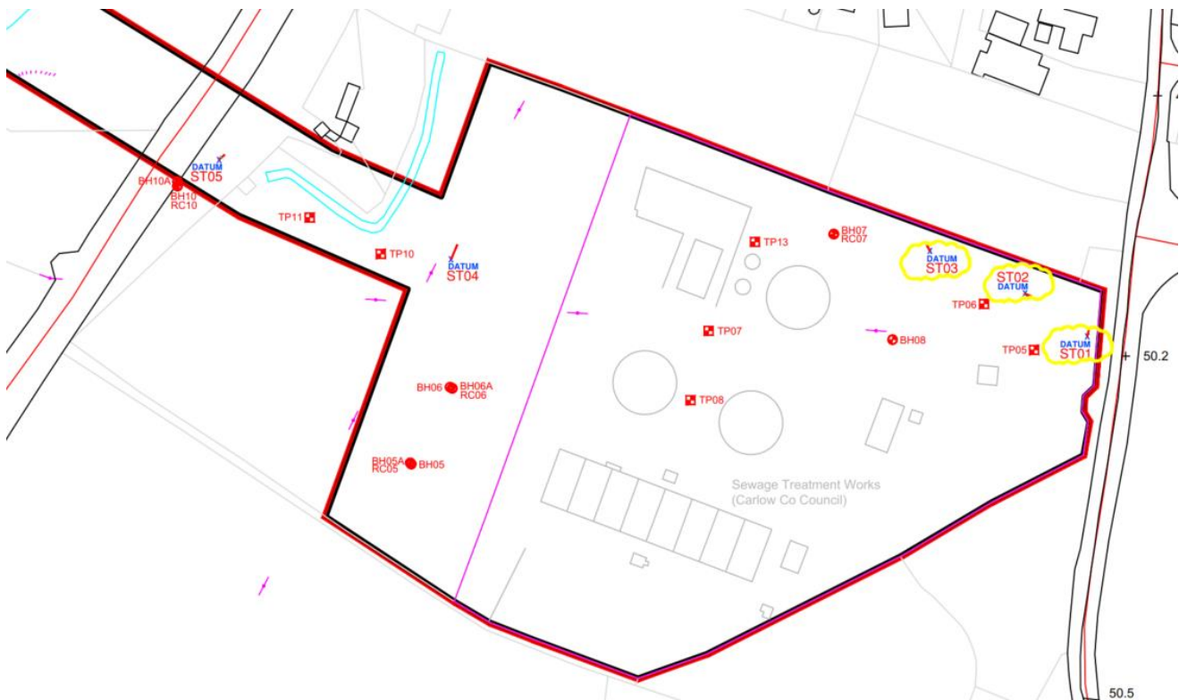
Figure 3 - Mortarstown WWTP GI locations
